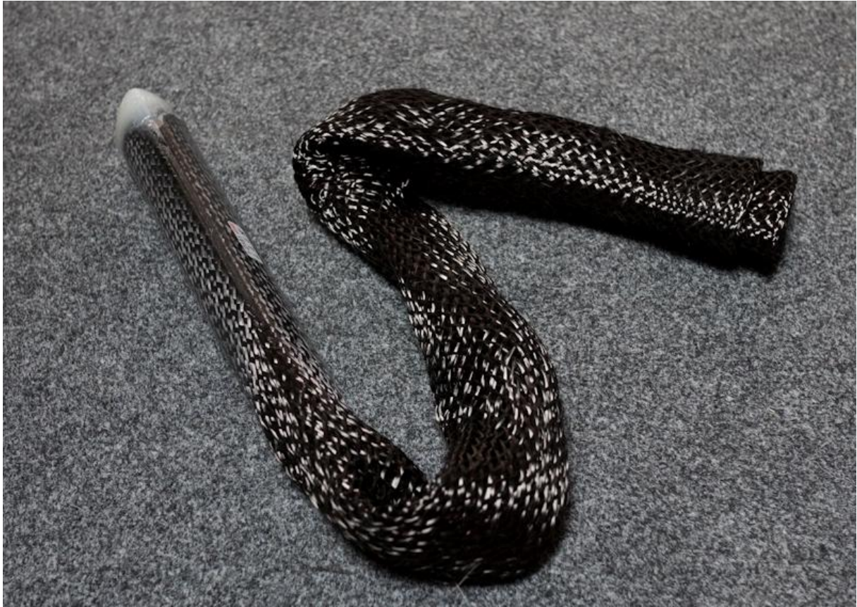
This is what a carbon weaved tube looks like with half of it resin treated and the other half without treatment. It's just a flimsy sock until it's hardened with resin.
